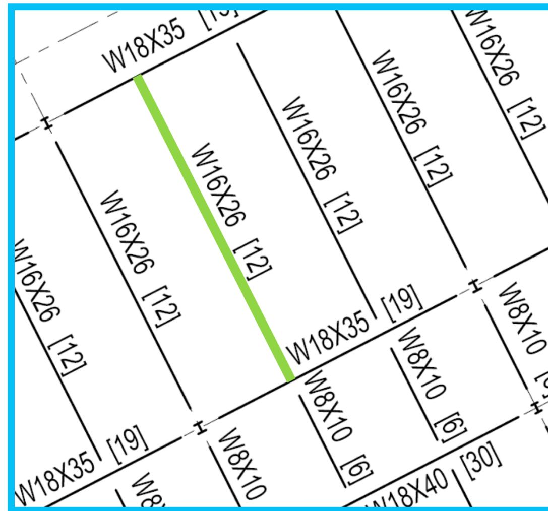
Typical Composite Beam Design (1<sup>st</sup>/2<sup>nd</sup>/3<sup>rd</sup> Floor Small Classroom)
